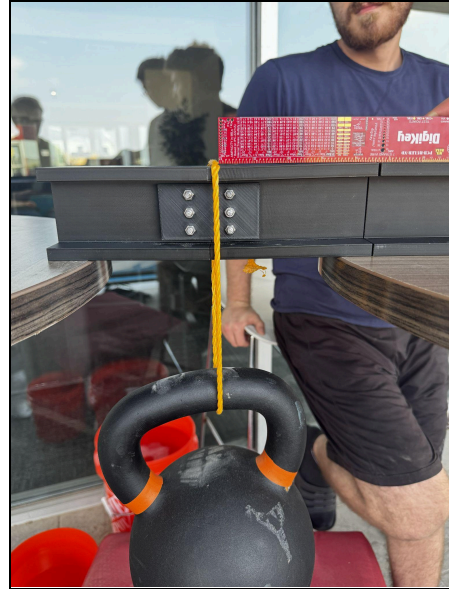
Figure 7: Midspan deflection of D2, loaded parallel to web
