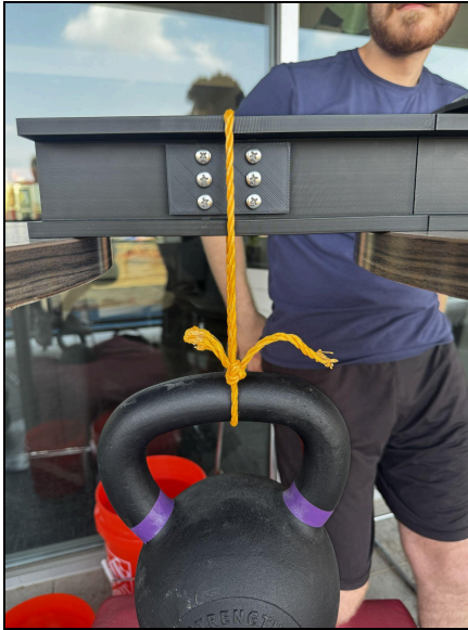
Figure 6: Design 2, loaded parallel to web
